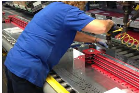
BEFORE: Using an incorrect tool to perform job tasks can lead to awkward postures and excessive exertions.
